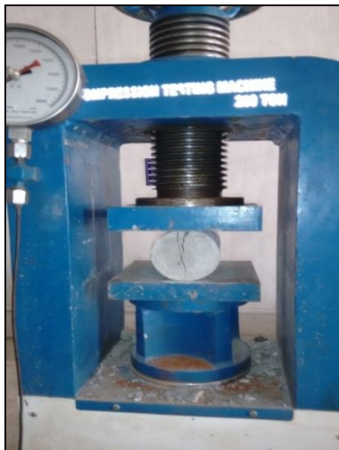
Figure 4. Split tensile test
